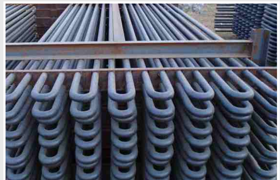
Super Heater Coils
