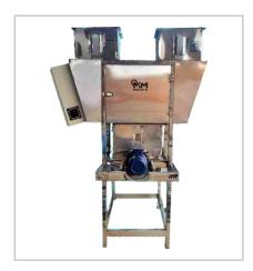
Robust Technology to blending fortified rice kernels to rice in an accurate and cost effective way. This is a multipurpose machine. This product can also blend two variety of broken rice with head rice in exact pre defined ratio.
