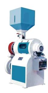
Rice Silky Polisher Machine is designed to gently polish the surface of the grain. Mixture of air & water is sprayed into the polishing chamber like a mist by means of a special atomiser. The use of water gives the output grains a shiny surface. It is suitable for:
